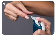
Remove the test card by sliding forward with your index finger and discard. Do NOT reuse Test Cards.
